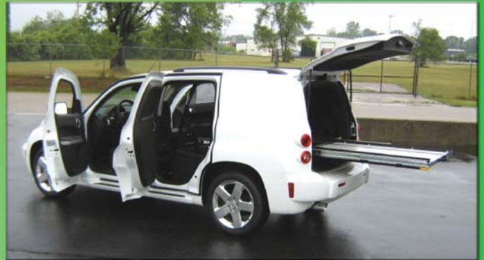
Pull Out Shelf for Ergonomic Lifting of Parts/Merchandise with Secure Latching Mechanism for Safety and Security.
