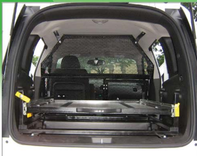
Bulkhead Barrier for Driver Safety and Ladder Door
